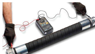
Hose assembly being tested with ohmmeter.
