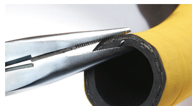
Pinching the staple into the tube wall.
